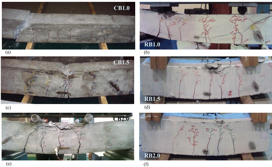
Fig.4: Crack patterns of beam specimens
