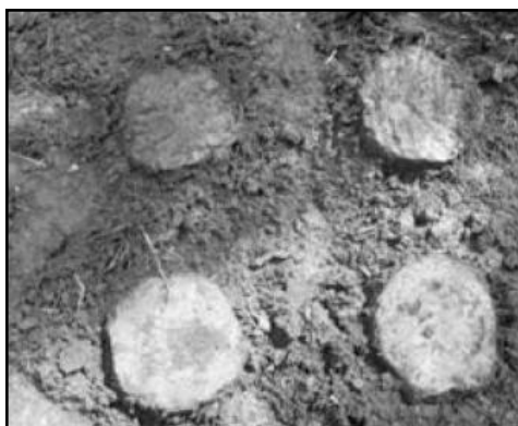
Fig.1: The layout of group PFA column-treated peat after 28 days (Islam & Hashim, 2010)
