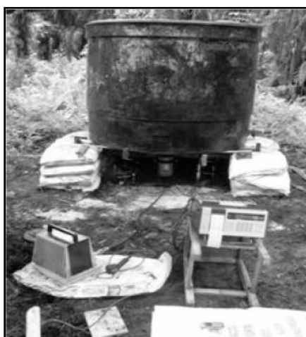
Fig.2: Layout of the static loading test (Islam & Hashim, 2010)
